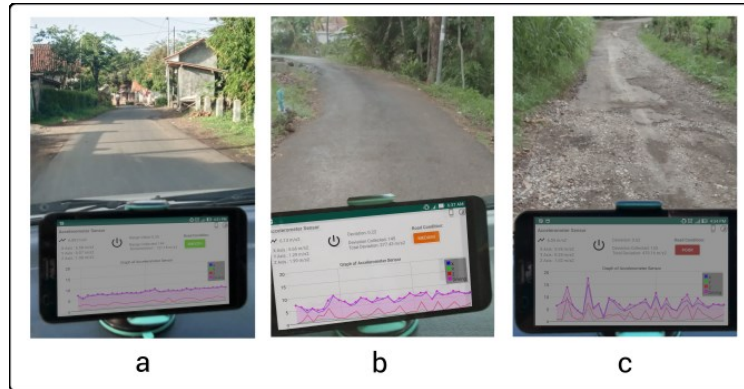
Figure 8. An Implementation of Road Conditions Analysis within a car: (a) Smooth Condition; (b) Medium Condition, and; (c) Poor Condition.
